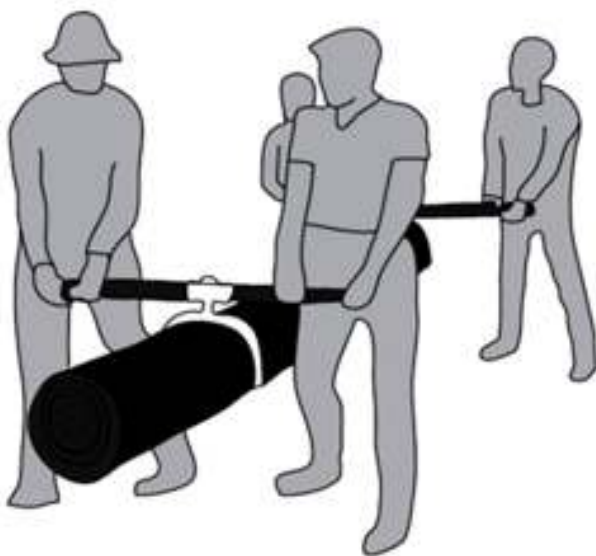
Figure 14: Tongs for log-lifting in a four-man team.
