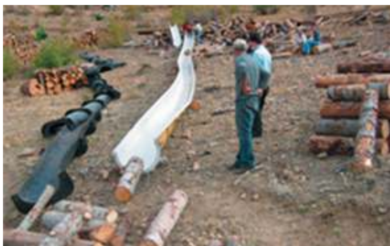
Figure 4. Comparative log line testing of locally manufactured log lines in Turkey (Acar, 2005)
