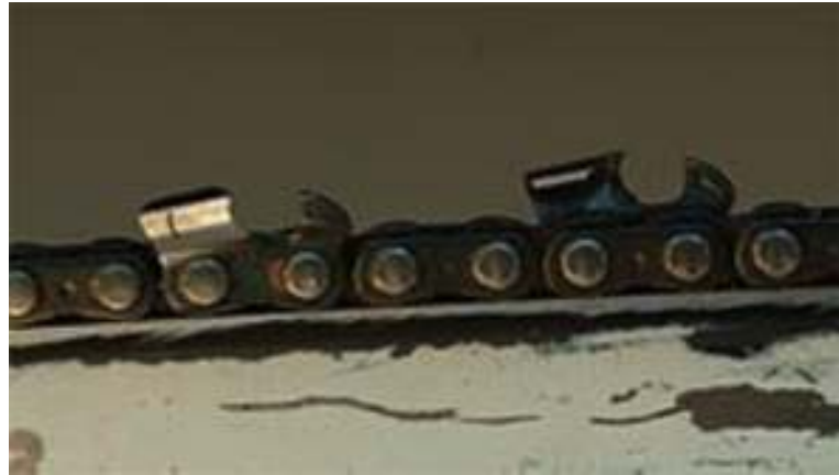
Figure 4. Chain on guide bar
