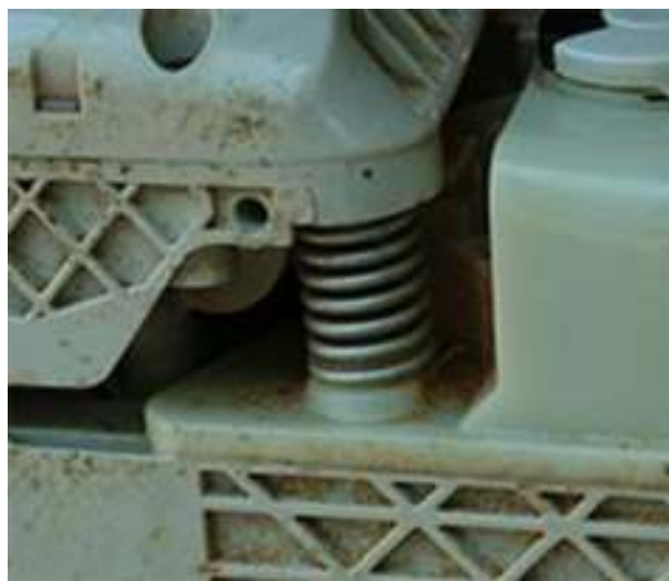
Figure 9. Metal spring anti-vibration system.
