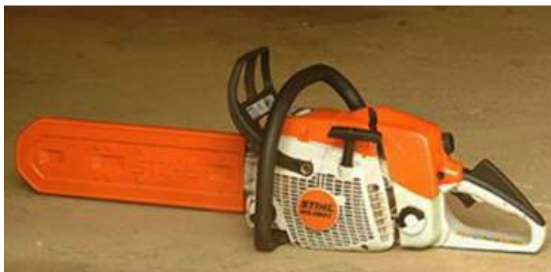
Figure 1. Chainsaw with protective scabbard over the bar and chain
