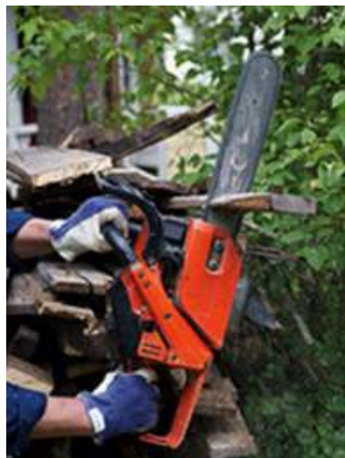
Figure 10. Rear-handled chainsaw used with a two-handed grip
