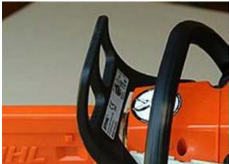
Figure 5. Front hand guard and a chain brake lever
