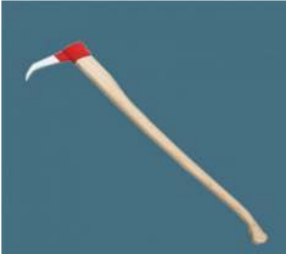
Figure 1. The sappie – the basic tool for manual downhill drifting
